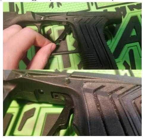
4) Make sure that the Pin is flush with the Plastic and Put all of the original adjustment screws into the New trigger and Adjust them to your liking and Enjoy!!
