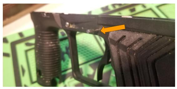
3) Install New Trigger and put the Pin back in the same way it was taken out.
