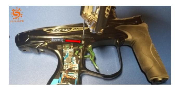
6. Once the trigger is installed and is catching when pressed or not sensitive you may need to rock the trigger left and right a couple times to free it.(one time thing and probably will not be needed)
