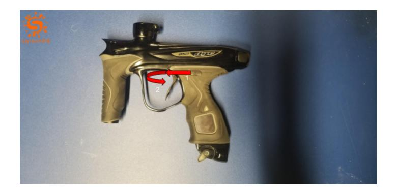
2. Take off these 3 parts: the screw holding in the trigger adjustment magnet, the trigger adjustment that is in between the trigger, the guide screw holding in the bearing.
