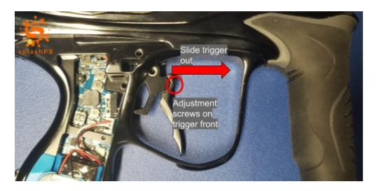
4. Get your new trigger and slide it in at an angle so that the top is just slightly in by the bearing. Then push the bottom of the plastic piece of the trigger up and slide it in.
