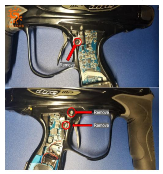
3. Slide out Trigger. If not coming out easy you may need to loosen adjustment screws for better angle.
